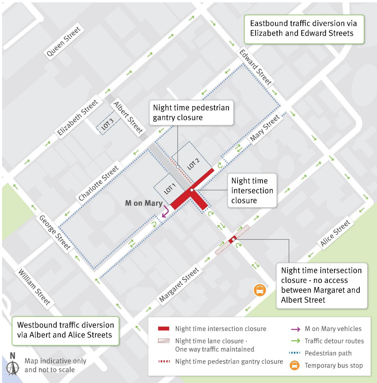
Above: Temporary night-time intersection closures of Albert Street at Mary and Margaret street intersections.
