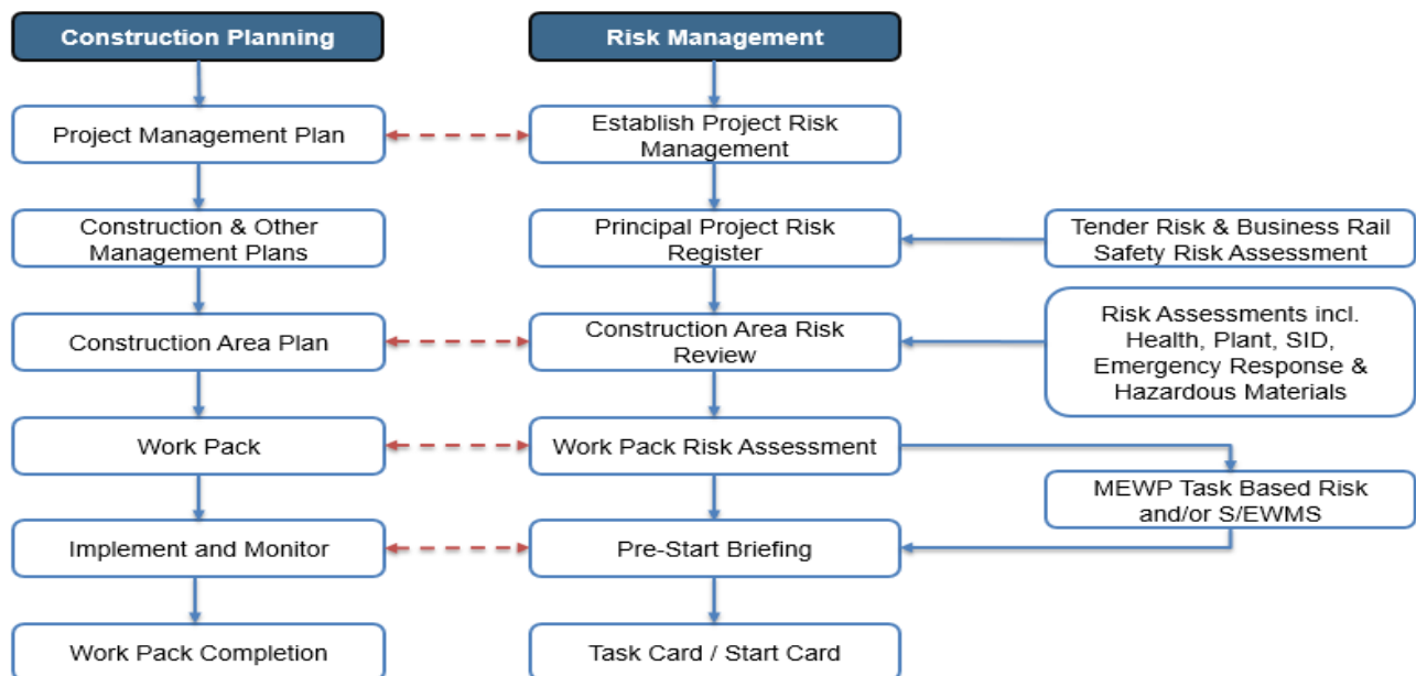
Figure 3 Construction Planning Process
