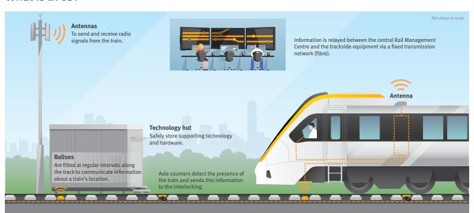
ETCS is an advanced digital signalling system. It's made up of a data radio system and fixed fibre transmission network that continuously relays information between the ETCS equipment trackside, on board trains and in the Rail Management Centre. With this flow of data, we know the position, speed, and direction of each train.
