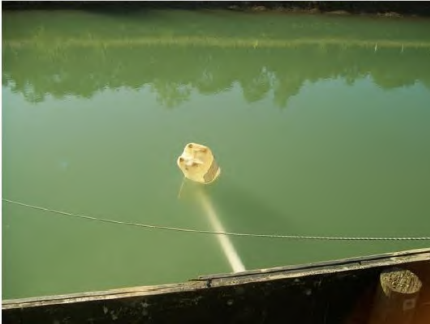
Floating inlet alternative to keep inlet above settled sediment
